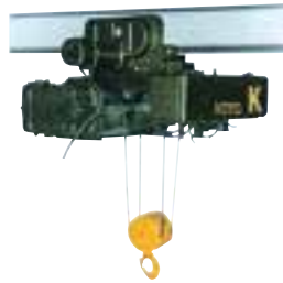
Low-head Motorized Traversing Hoist At the upper limit, the headroom (the distance between the outer bottom of the rail and the hook center) is minimized. (Suitable for a place with low ceiling)
