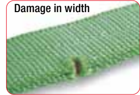
Damage in width
